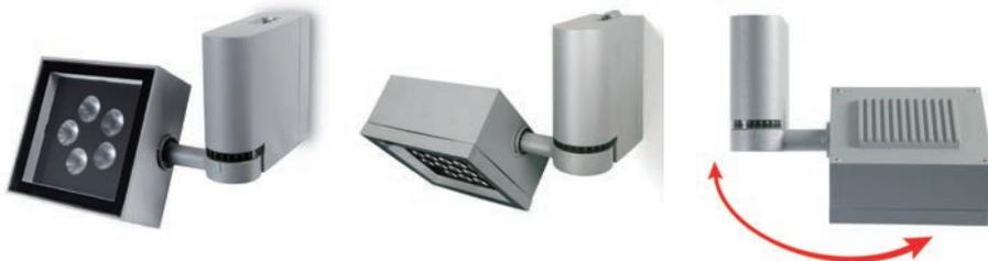
Two graduated rings precisely indicate the aiming angle of the head with a friction based mechanism which maintains the position, further secured by tightening the screws.
