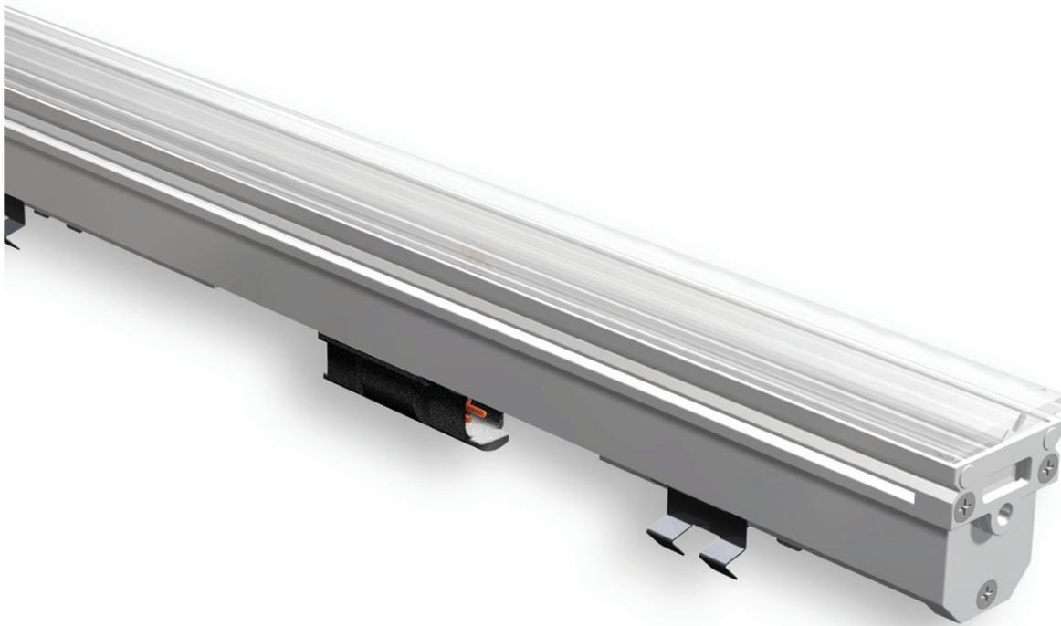
The walkable line which interprets space and volume. Cursus expresses with great effect LED homogeneous linear light. A range of four crystal perimeter-finished elements, aggregable linear fixtures complete with housings that can be loop-powered in only 5 seconds while maintaining the IP67 protection, with a thickness of only 55mm and a width of 30mm. Simple and easy mounting, with a wide range of accessories, floor and surface installation, make it a reference point for the market.
